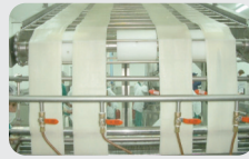
Cooling Steamed sheets are cooled through the cooling conveyor
