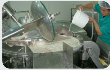
Mixing Mixing surimi and ingredients with silent cutter
